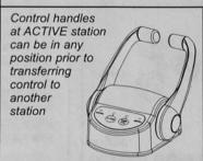
Control handles at "station taking control" MUST be in an appropriate handle position to transfer control to it
