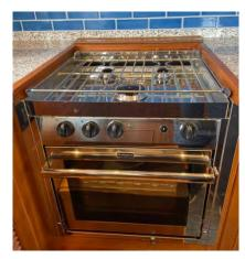
Caution: propane is heavier than air and will settle to the lowest points in a boat- the bilge. If a leak
