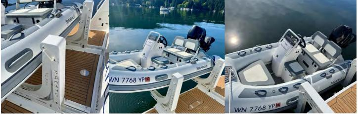
Tender floating free of lift with lines used to control. Lift fully lowered to allow positioning of the tender. Lift raised and in intermediate position. Secondary tie downs attached to lift and lift arms.
