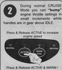
Mode you can "bump" engine throttle settings in small increments while
