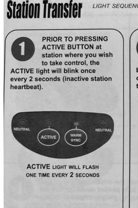
LIGHT SEQUENCE AT STATION TAKING CONTROL DURING STATION TRANSFER PROCESS
