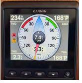
**MERCURY ENGINE MONITORING SYSTEM** - Starboard of the MFD. Easiest way to monitor engine fuel consumption. It takes approximately 1 minute to boot up and perform engine systems check when the ignition key is turned on. It is not a touchscreen. Use buttons to scroll up and down. The Home and Speed screens are the most useful.
