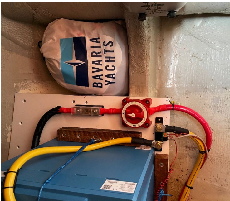
House battery on/off switch (leave on) located under forward berth, just forward of the battery. House battery monitor located above forward end of nav station. Charge battery no later than 13.0v or 20% state of charge.
