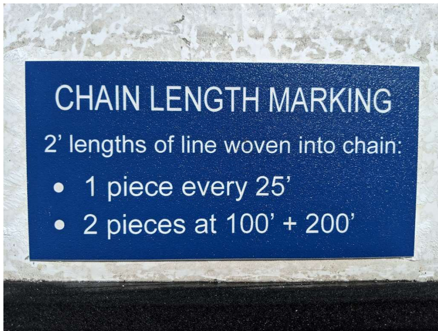
ANCHOR CHAIN PLACARD – ANCHOR LOCKER LID
