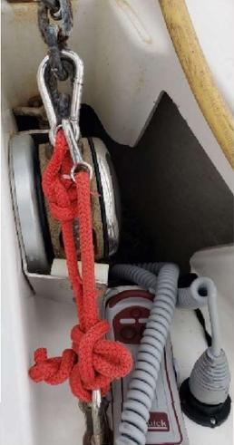
The **anchor tension line (snubber)** is red and used to keep the primary anchor chain taut and remove stress from the windlass when underway. **Do NOT use when anchored.**
