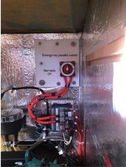
**Emergency panel switch connects house bank to the starter battery.** This is in the event the start bank is dead. The switch is on the port side back wall of the engine compartment. Once the engine has started, turn the switch back to the off position and proceed with motoring.
