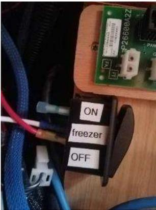
**You can turn off the freezer** using a switch behind the settee cushion forward of the navigation station. Remove the back cushion and look to the right.
