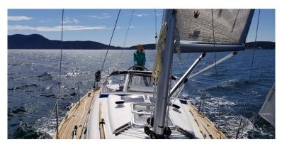
The boom / mainsheet can be stored to the side when motoring or at anchor. The sprayhood can be rolled away neatly into a protective cover (see sailing section). The washboards store in the cockpit locker. Fenders can be stowed in the dinghy when underway.
