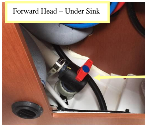
Valves to drain holding tanks overboard
