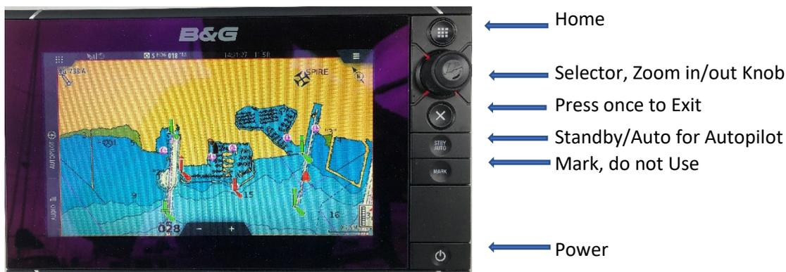
**Finding Home Page/Main Menu:** After turning on the Power Key, hit the Home Key to find the Chart Plotter, Radar, and Tides functions. We recommend that you only use these three functions. The Autopilot is much easier to manage at the small control at the starboard helm. Guests are asked not to set waypoints and routes because the “drift” impact of Pac NW currents require constant attention.
