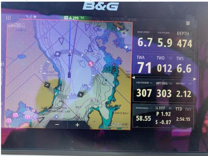
If you pan and scroll to look at different portions of the area, simply hit “Clear Cursor” in the lower right-hand corner to bring the vessel back to the center of the chart. Note that the Blue Line is where the vessel is pointed. The Red Line is the Course Over Ground (COG) line. This is where the vessel is actually going taking in to account current, leeway, etc. **If your blue line shows a clear path but your Red Line is crossing rocks or other hazards, you need to take action.**
