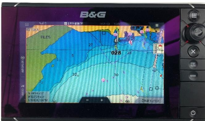
**Depth Sounder:** The B&G unit’s measurement is set in feet. There is no “Keel Offset”. That is; the transducer is set to where it is. The bottom of the hull. With a draft of 7 feet, If you’re reading 5 feet of depth, you’re likely aground.
