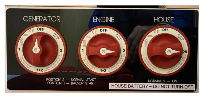
**Normal Conditions:** Generator in the No. 2 position (**different from what is shown in picture!**), Engine in "No. 2" position, and House in the "On" position.
