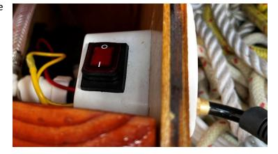
b) Get the washdown hose ready – inside the exterior bow locker. Very important to clean the chain before it goes into the chain locker. Helps prevent tangles next time lowering. The washdown pump switch is also inside the exterior bow locker, up high at the aft end – see photo above.
