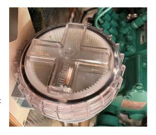
• Inspect the raw water strainer for debris. In case of an engine overheat alarm, check for eelgrass
