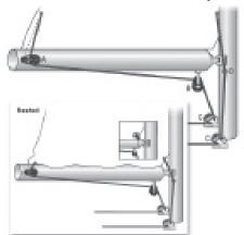
This diagram shows a common reefing system using two lines. Lines can cleat on the boom and mast or be run back to the cockpit. Courtesy www.Harken.com
